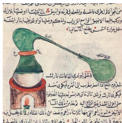
Figure 6 - Drawing and description of Alembic by Jābir ibn Ḥayyān from eighth century (Photo sourced from Wikimedia and is in public domain)
